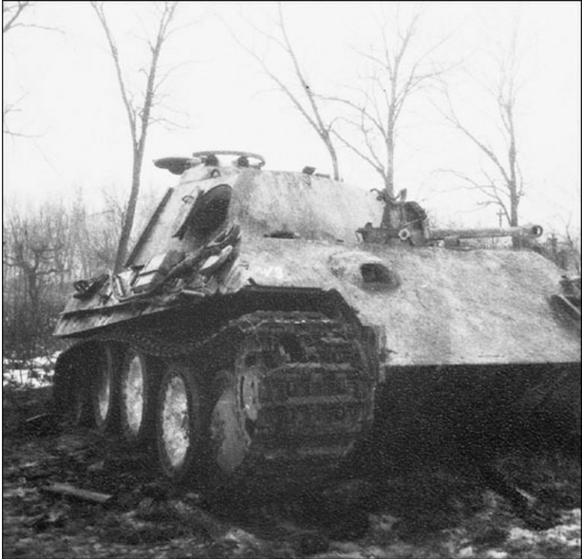
The same machine as in the previous photograph, seen from a different angle. It is clearly visible that the tank is lacking a Zimmerit coating.
