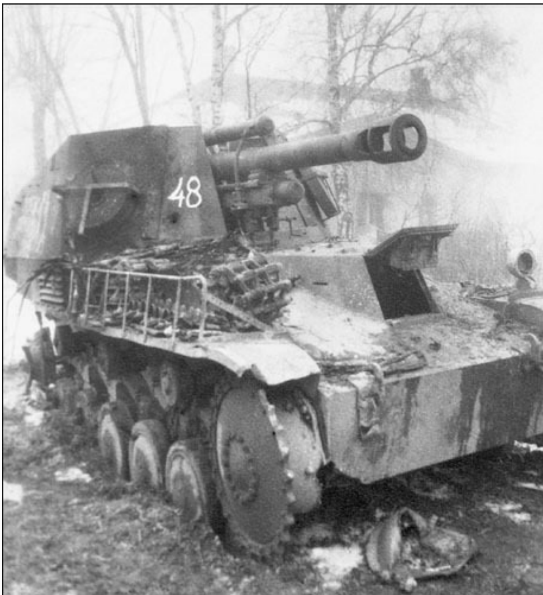
An abandoned Wespe self-propelled howitzer. The tracks have been removed, most likely as a matter of convenience for towing.
