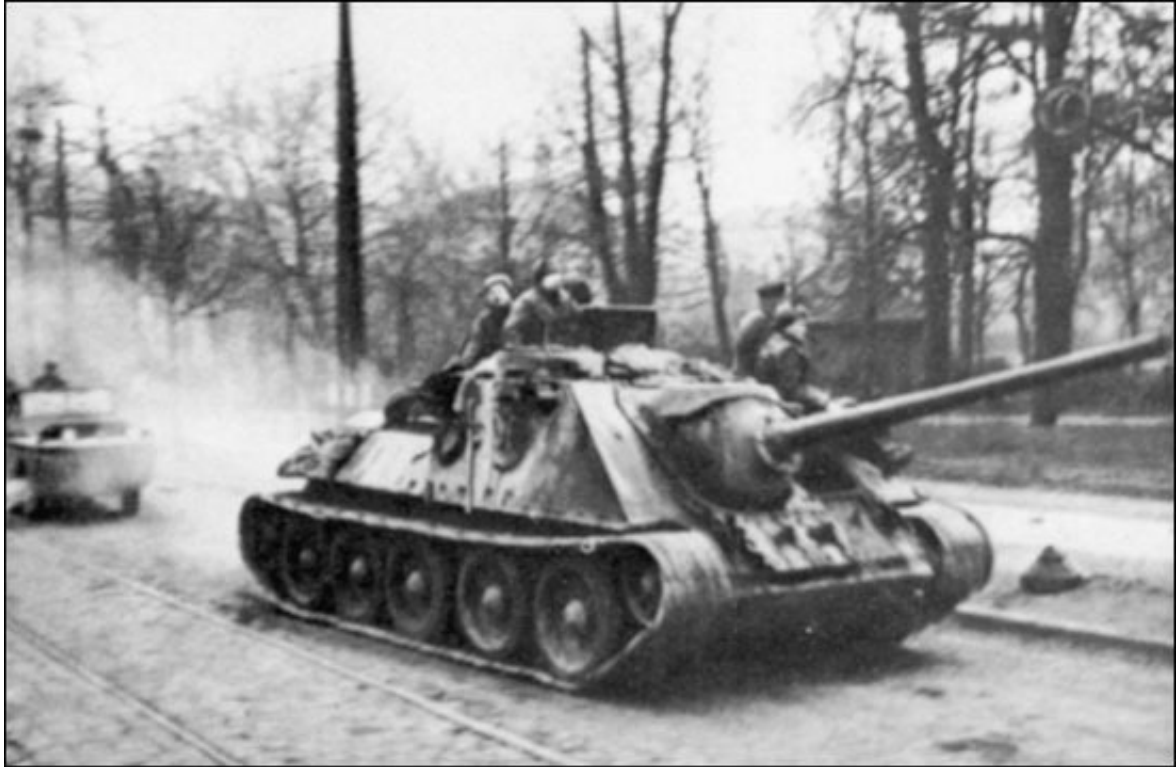
An SU-85 on the move. These self-propelled guns were used as tank destroyers, but with the widespread introduction of the T-34/85 tank they lost their significance, since they were no longer better armed than the T-34 and lacked turrets.
