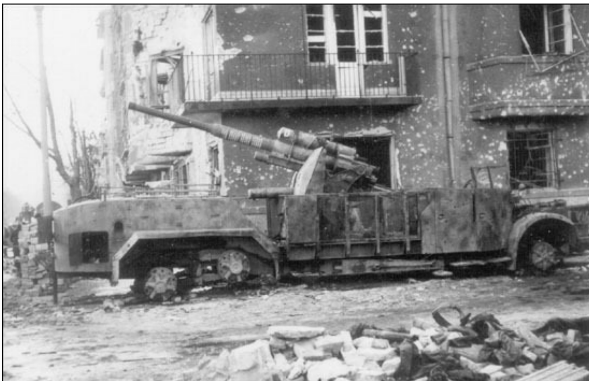
An 88mm gun mounted on the chassis of a Bussing Nag on a Budapest Street. Note the white rings
