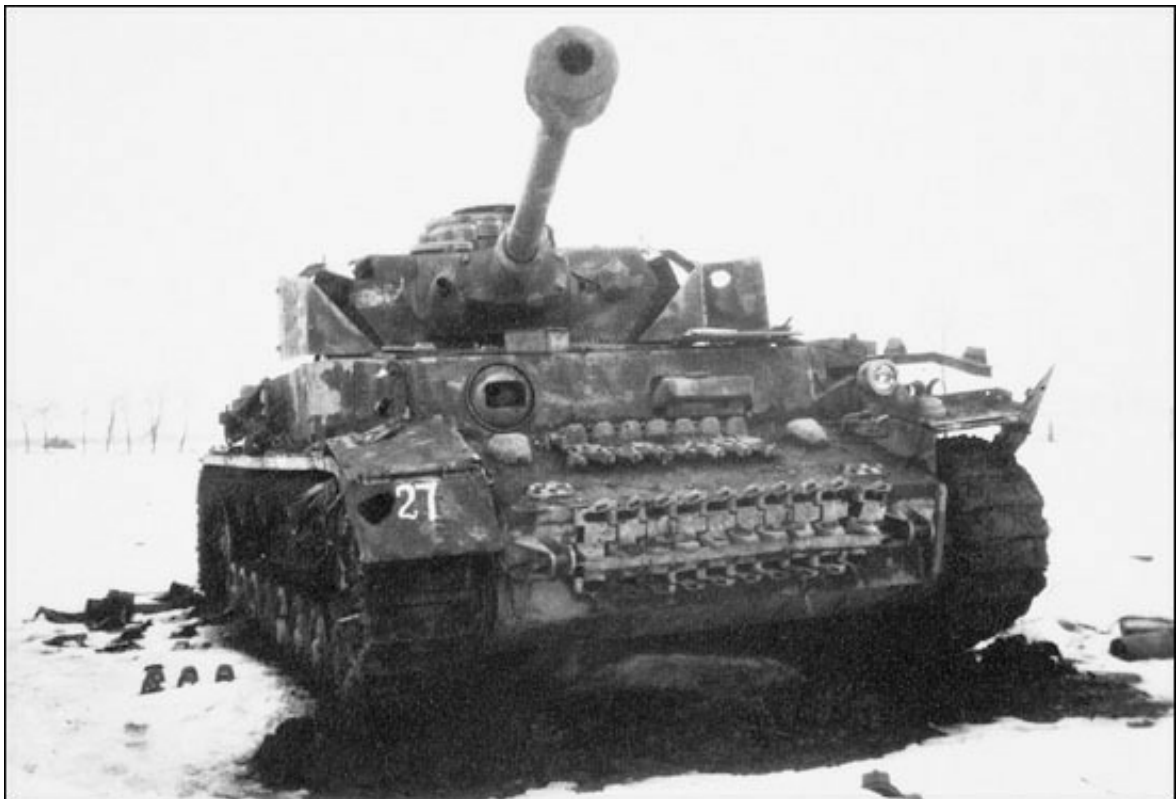
A knocked-out Panzerjäger IV tank destroyer. Note the Zimmerit coating covering the armor.
