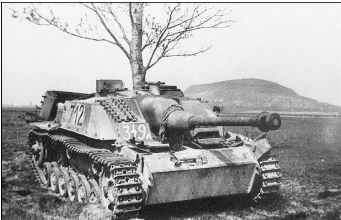
A StuG 40 self-propelled gun abandoned on the battlefield. The machine is fitted with a Saukopf gun mantlet and bears the tactical number “712”.
