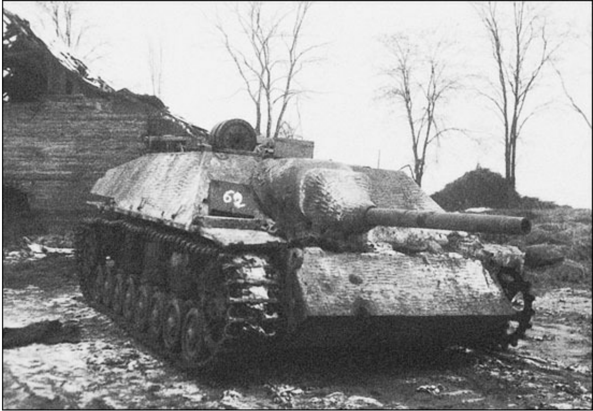
A knocked-out Panzerjäger IV tank destroyer. Note the Zimmerit coating covering the armor.
