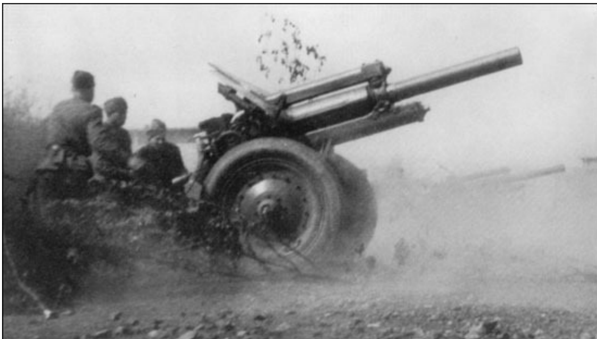
A divisional M-30 Model 1938 122mm howitzer in action. By 1945, these guns made up the bulk of the artillery in the Red Army's rifle divisions.
