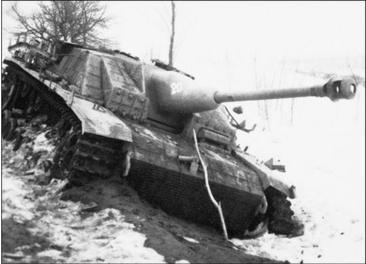
This bogged down StuG 40 assault gun is fitted with a Saukopf gun mantlet and has a Zimmerit coating.
