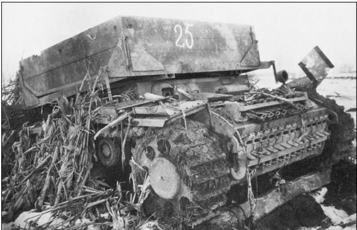
A close-up view of Totenkopf 's knocked-out Tiger tank. The shell hole in the front armor plate is clearly visible. (TsAMO)
