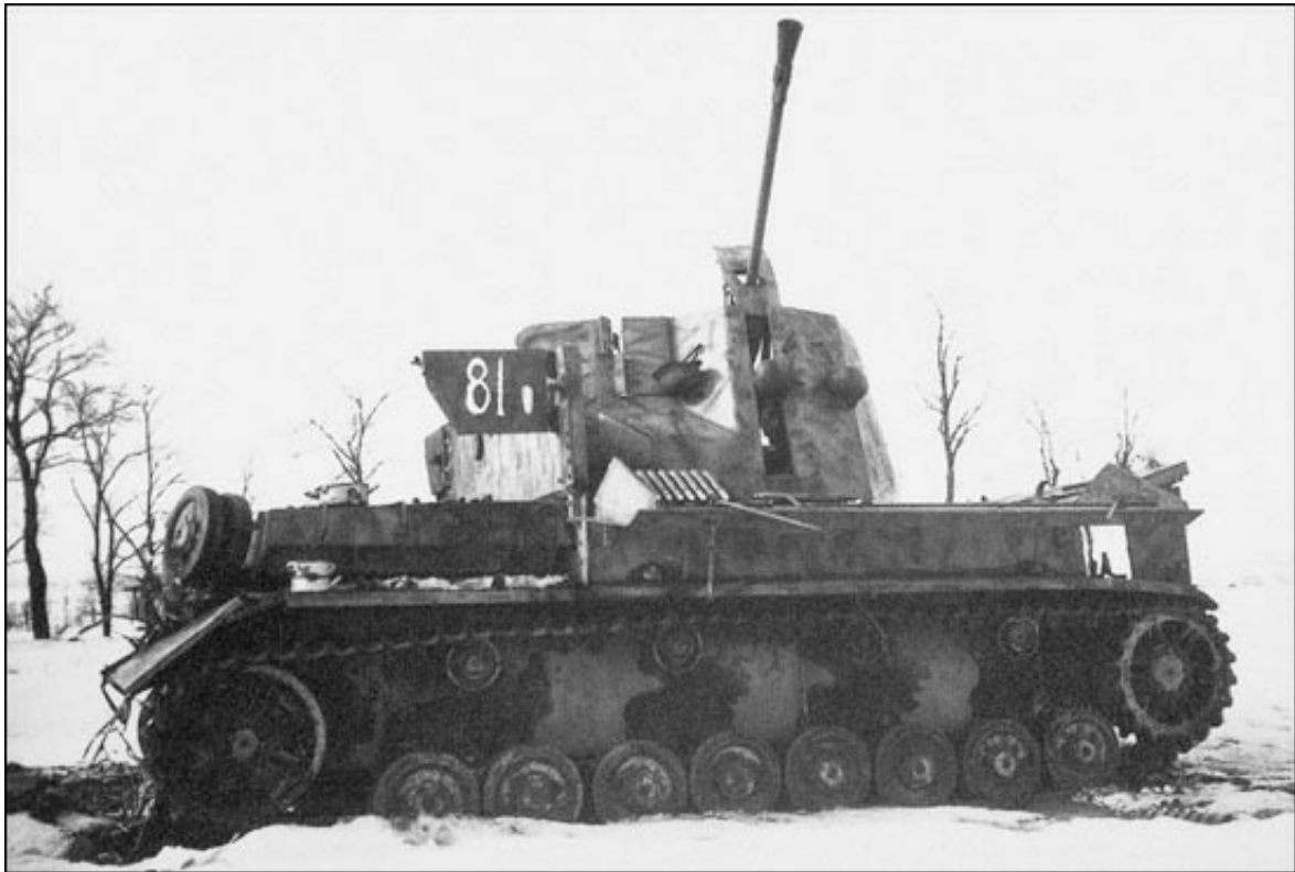
An anti-aircraft Flakpanzer IV Möbelwagen with the 37mm Flak 43 cannon, February 1945, Budapest area.
