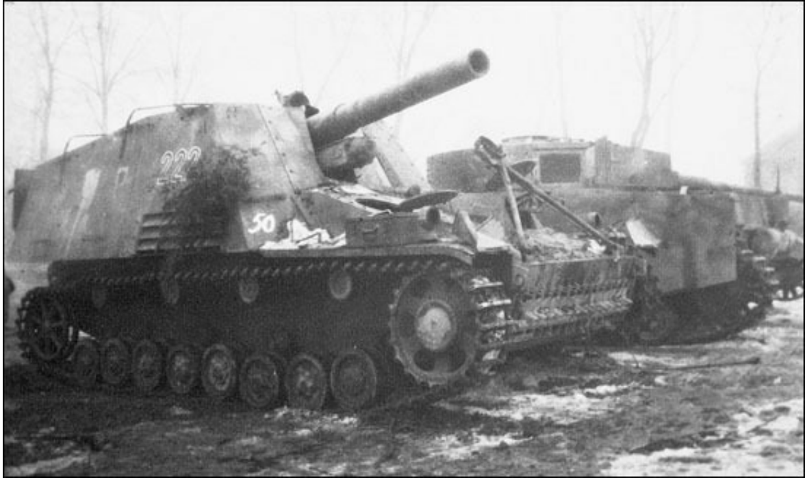
German armored vehicles seized by Soviet troops: A Hummel self-propelled howitzer and a Pz. IV tank. Note the arcs welded onto the Hummel's fighting compartment to provide for a tarpaulin covering.
