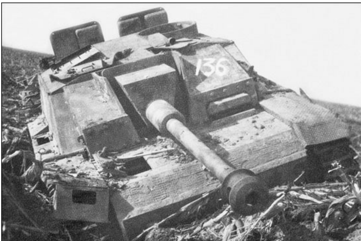
A StuG 40 self-propelled gun that has become immobilized in the mud and was abandoned by its crew. The number "136" was left there by the Soviet inspection team. Note the waffle-pattern Zimmerit.
