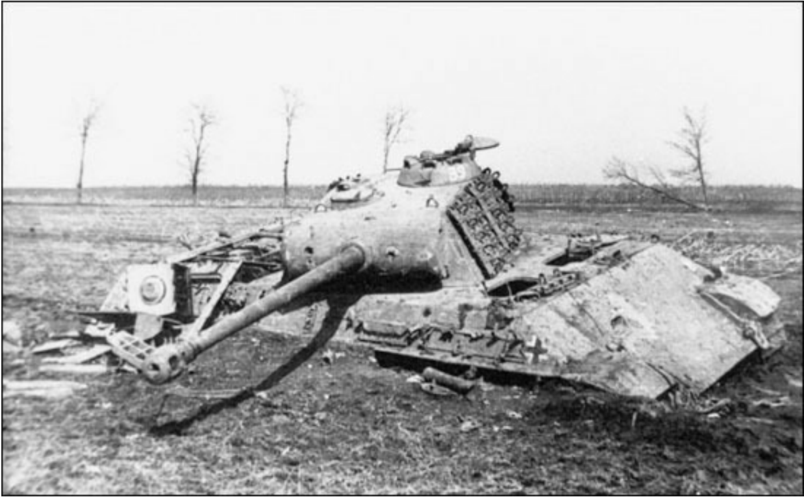
A deeply mired Panther, abandoned by its crew. Spare track sections have been mounted on the tank's turret as supplementary protection.
