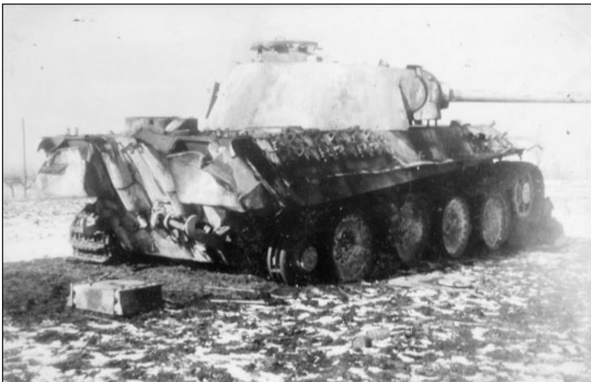
A burned-out German Panther Ausf. G tank. The tank has plainly “settled” as a result of the collapse of the torsion bars due to the fire. (TsAMO)
