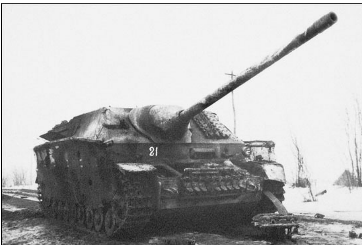
A Jagdpanzer IV/70(A) tank destroyer, knocked out in the area of Lake Balaton. The machine has Drahtgeflecht [wire mesh] Schürzen side skirts and is wearing the remnants of winter camouflage.
