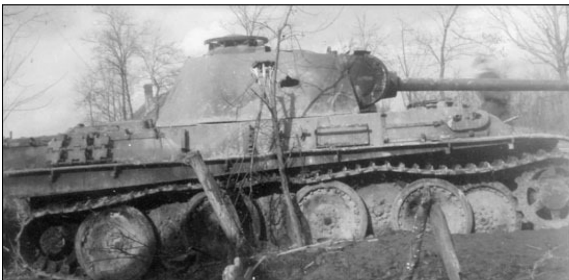
A knocked-out Panther, Hungary, January 1945. Shell holes are clearly visible in the side armor of the turret. (TsAMO)
