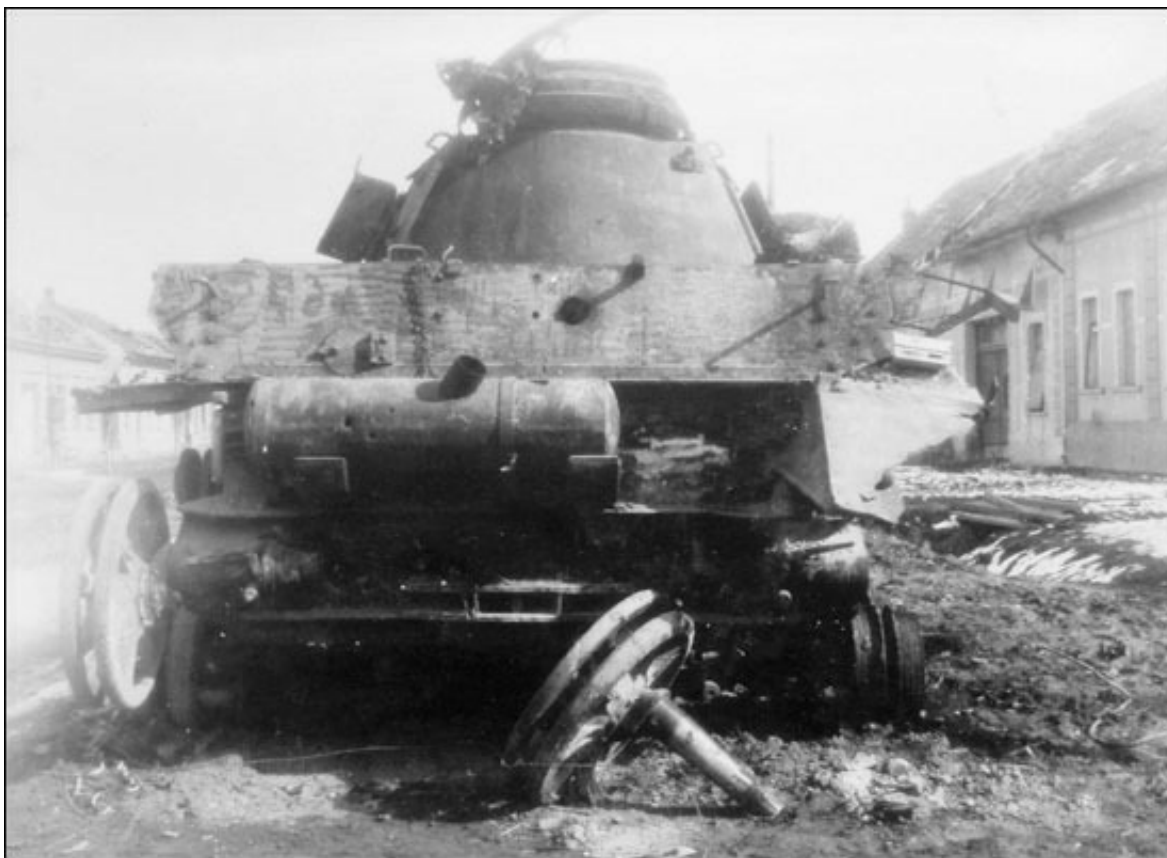
A Pz.Kpfw.IV tank knocked out by a shell hit in the rear of the hull. (TsAMO)
