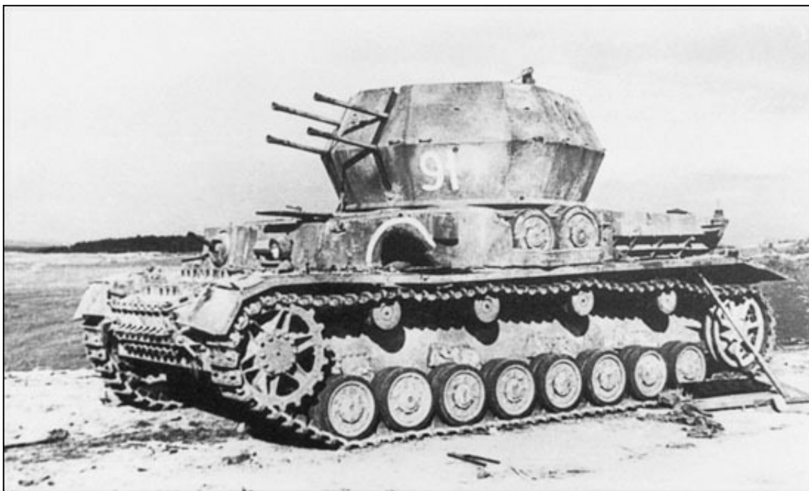
A Flakpanzer IV Wirbelwind self-propelled anti-aircraft vehicle, destroyed by the direct hit of a large caliber shell. The gaping hole in the side of the hull is clearly visible.
