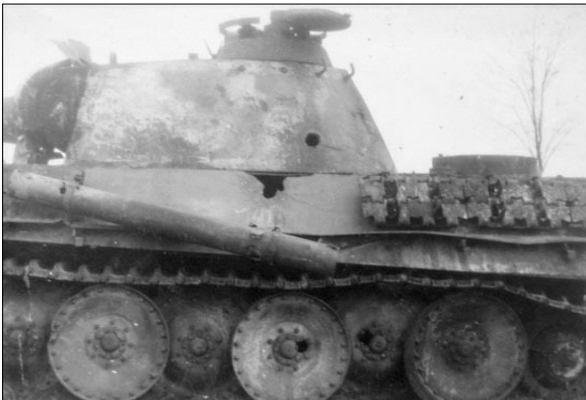
A close-up view of the flank of the tank in the preceding photograph. Plainly, it has been literally riddled with anti-tank rounds. Note the roller wheels that have been shot through by armorpiercing shells.
