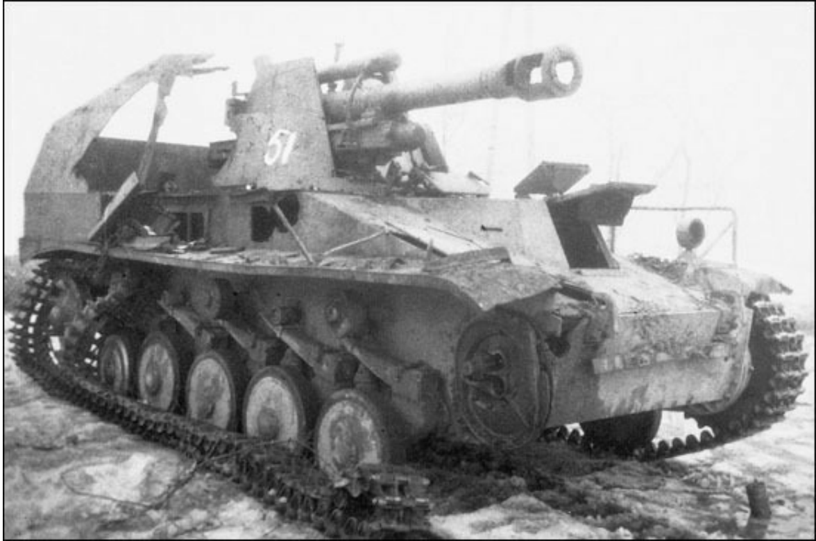
Yet another knocked-out Wespe self-propelled howitzer. These self-propelled guns, possessing armor protection against shell fragments and firing from covered positions, were a hard nut to crack, and only a direct hit could knock them out.
