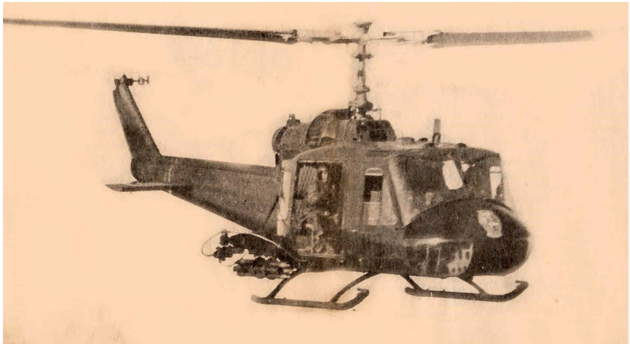
UH-1C (Charlie Model) gunship equipped with rockets and miniguns.
