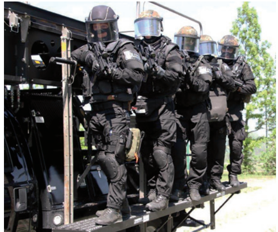
Austrian EKO Cobra operators travel to a target on the running boards of a Patriot 3 MARS intervention vehicle. The MARS system allows running boards to be raised or lowered to deliver assaulters at the correct height – for example, at window-level for a bus assault. These officers carry the 9mm B&T APC9 sub-machine gun. The second from the right, armed with a Glock pistol and wearing heavier armour, is probably the 'shield man' who will be the first through the door. (Photo courtesy BM.I/Polizei)
