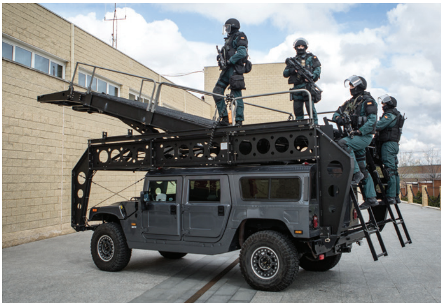
An assault team from the Spanish GEO during an exercise in 2016. The vehicle is the so-called 'Spanish Humvee', the URO VAMTAC, fitted with a MARS adjustable ladder unit. The rifleman (centre) has a 7.62mm HK417 with a thermal day/night sight partnered with a telescopic optic; the assaulters carry MP5s with angled stocks to accommodate their visors. (Photo Pablo Cuadra/Getty Images)
