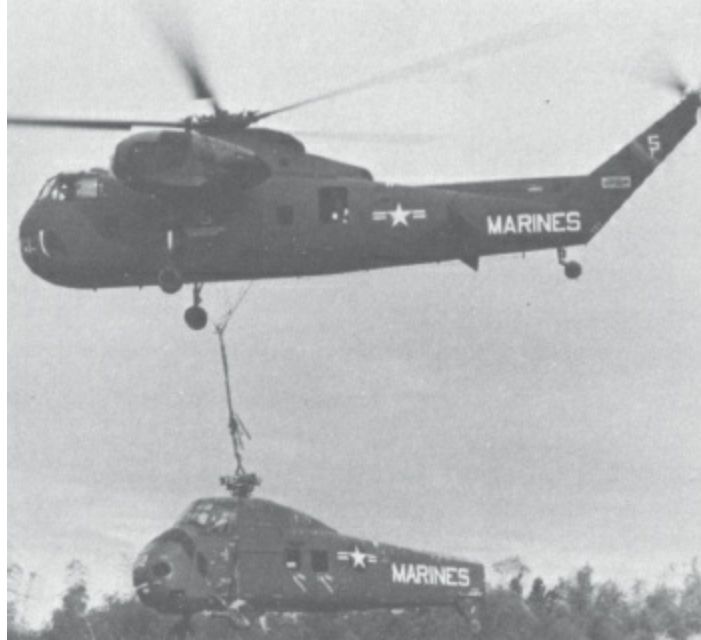
A Sikorsky CH-37 twin-engine helicopter is seen recovering a damaged UH-34. The CH-37 was used primarily to airlift supplies and equipment.
