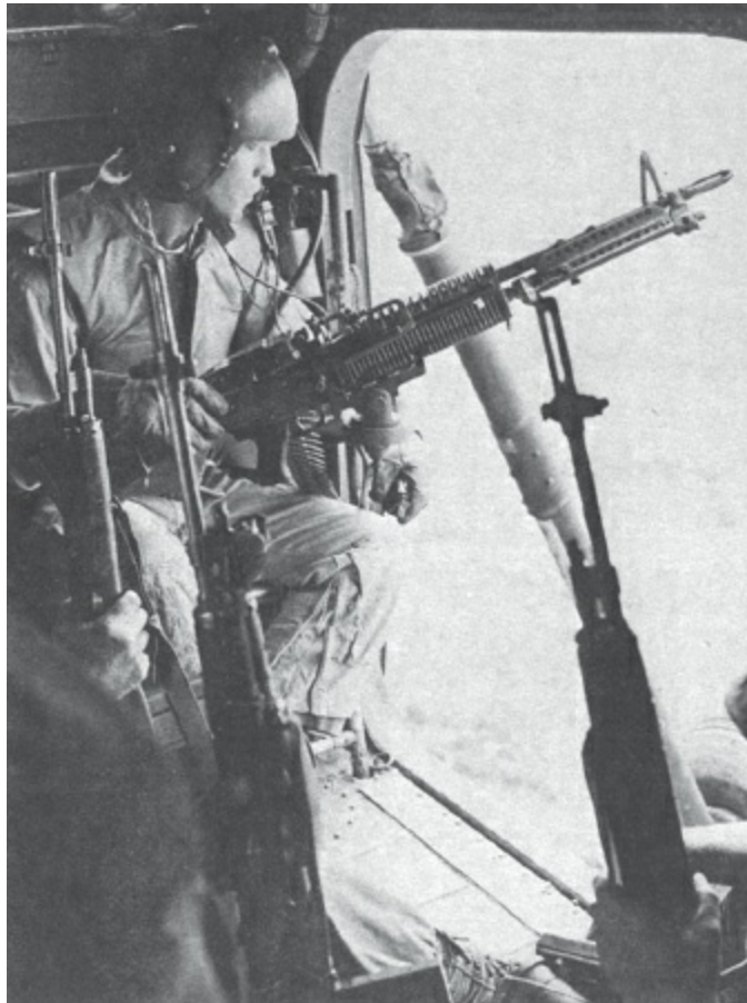
A UH-34 door gunner mans an M60 7.62mm machine gun. The door-mounted machine gun improved the helicopter's firepower protection.
