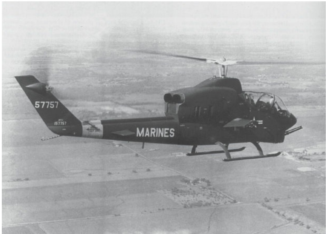
The Bell AH-1 Super Cobra is a twin-engined attack helicopter. It was initially developed in the mid-1960s for the U.S. Army and later modified to meet Marine Corps requirements. Marine AH-1J Sea Cobra arrived in Vietnam for evaluation in February 1971. It carried a three-barrel 20mm cannon in its nose turret, capable of firing 750 round per minute.
